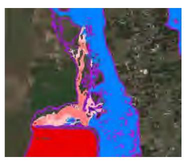
Figure 5.9 Developed 100 yr Flood Afflux 360min
