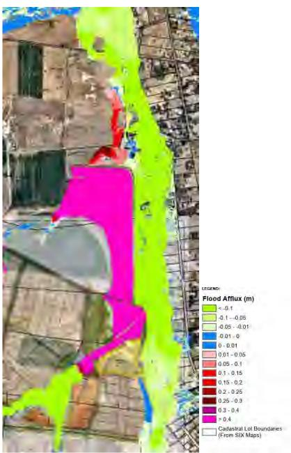
Figure 10: Flood afflux with temporary farm dam
